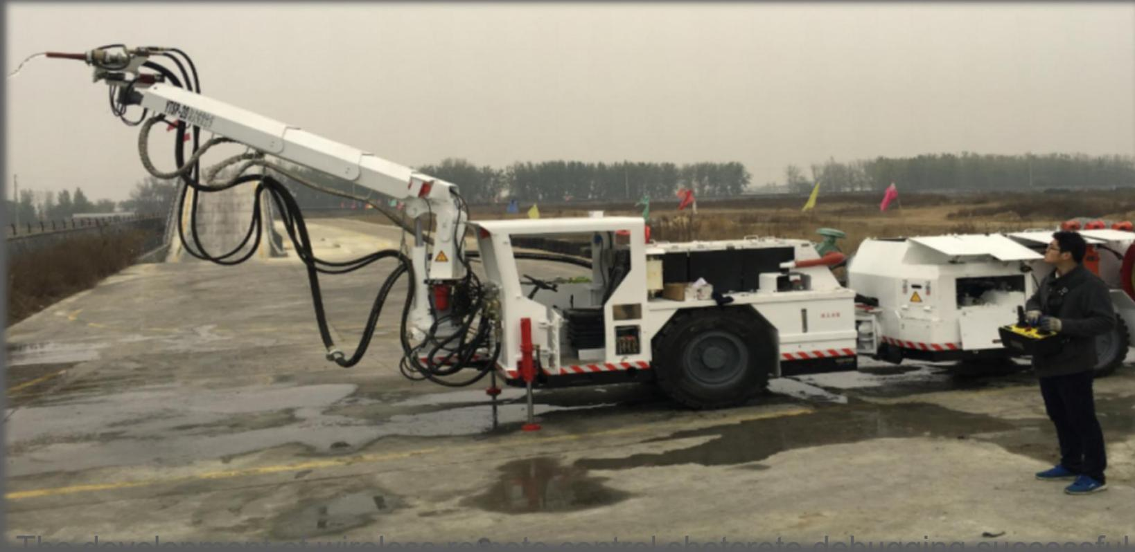
The development of wireless remote control shotcrete debugging successful
